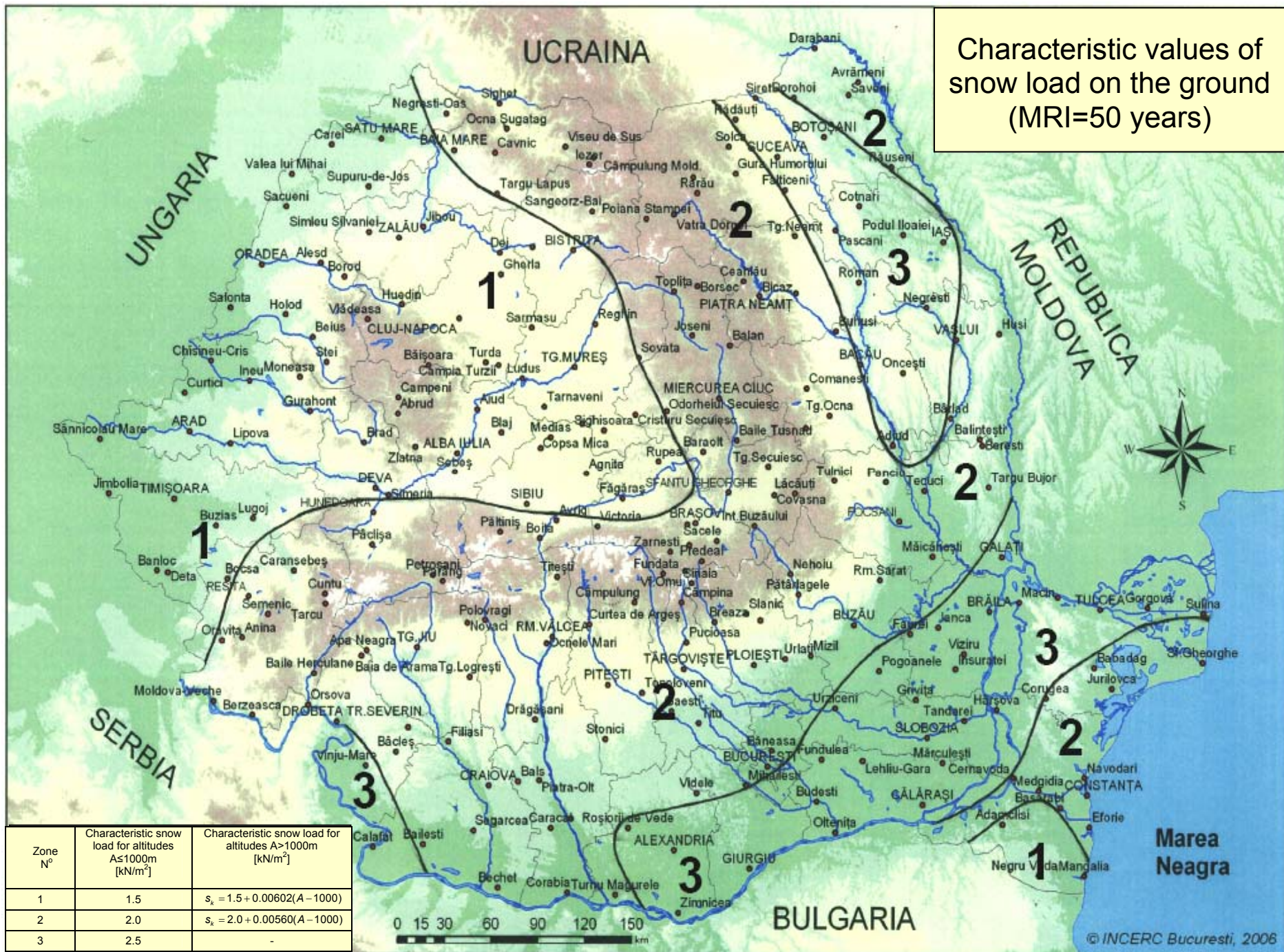
Figure NA.1 – Romanian snow map of characteristic snow load on the ground referred to mean recurrence interval equal to 50 years
